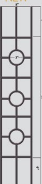
HF 9.4.44 Ends : 1/2" Sq. Height: 46" Wt. 4.9 lbs. TUBULAR (Rake)
