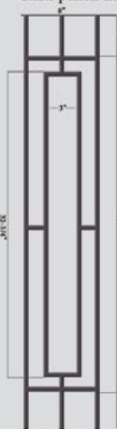
HF 9.4.1 Ends : 1/2" Sq. Height: 44" Wt. 4.4 lbs. TUBULAR (Level)
